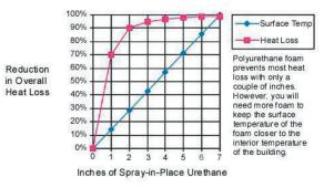
The graph shows that 70% of heat loss from conductance is stopped by a one inch thickness of spray-in-place urethane foam. Remember we are going to stop nearly 100% of the heat loss from
